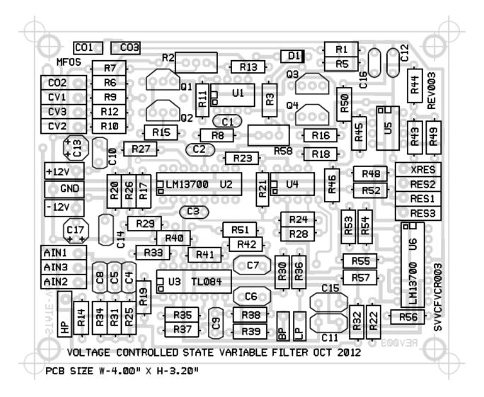
State Variable VCF 12dB/Octave With VC Resonance PCB Parts Layout (Parts Side Shown)
