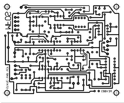
State Variable VCF 12dB/Octave With VC Resonance PCB Top Copper(Parts Side Shown)
