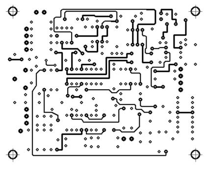
State Variable VCF 12dB/Octave With VC Resonance PCB Top Silk Screen
