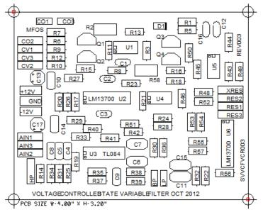
State Variable VCF 12dB/Octave With VC Resonance on the Breadboard
