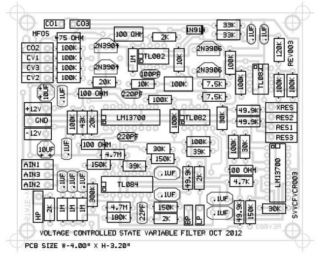
State Variable VCF 12dB/Octave With VC Resonance PCB Bottom Copper (Parts Side Shown)
