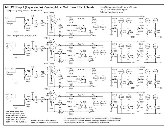
In the *Stereo Mixer* there are four mono input channels and four sets of stereo line inputs. Each mono input consists of a level pot, capacitively coupled to a buffer amplifier. Channel one for example has R2 (100K audio taper pot) as the input level control. The wiper is connected via C1 and R3 to U1 (TL071 low noise op amp) which provides a gain of 10.
