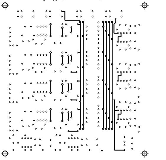
Stereo Mixer PCB Top Copper(Parts Side Shown)
