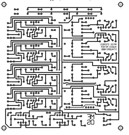
Stereo Mixer PCB Bottom Copper (Parts Side Shown)
