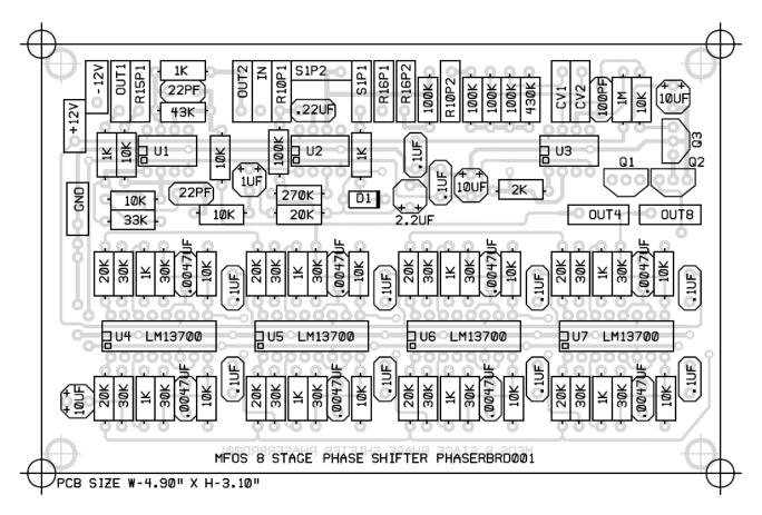
**Eight Stage Phase Shifter PCB Bottom Copper (Parts Side Shown)**
