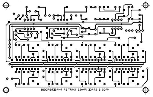
**Eight Stage Phase Shifter PCB Top Copper(Parts Side Shown)**
