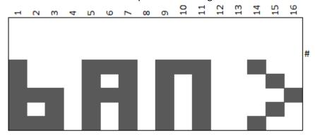
After releasing the Sequence Cmd button, the display shows the value screen to enter the bank number 01-03. Press the Value control knob to enter the bank number selected.
