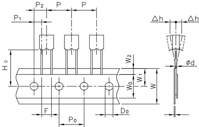
**Figure 2 – Lead Space 7.5 mm**
