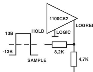
**Fig.9** Diagram with divider at the input for setting the threshold, threshold voltage  $U_{\pi} = - 4V$ .
