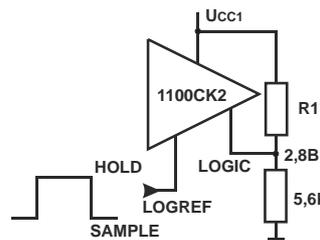
**Fig.5** TTL and CMOS levels, sample low, threshold voltage  $U_{\pi} = + 1.4V$ .
