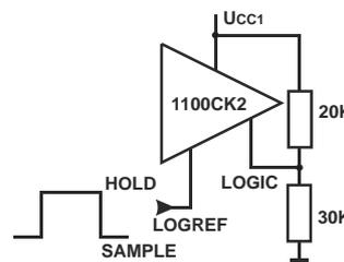
**Fig.6** CMOS levels  $7V \leq U_{OH} \leq 15V$ , high sample, threshold voltage  $U_{\pi} = 0,6U_{CC1} + 1,4V$
