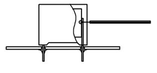
Temperature monitored inside the capacitor.
