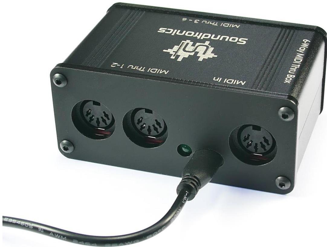
That's it, you are ready to go. The Thru Box draws very little power just 10-30mA and the adaptor is also very efficient so energy consumption is negligible. Please note that the power supply must be 5V dc regulated, damage to the Thru Box electronics may occur if an incorrect voltage is used.
