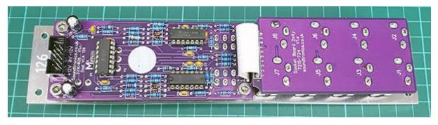
Insert the chips into the sockets in readiness for testing.
