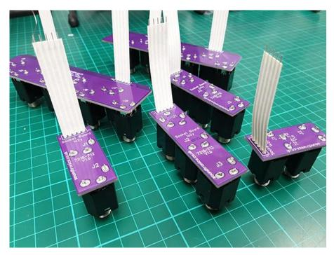
Step 3 – Soldering the jack socket PCB to the main PCB requires a bit of ingenuity. Really important is the orientation of the jack socket PCB in relation to the main PCB. The photo shows the correct way around.
