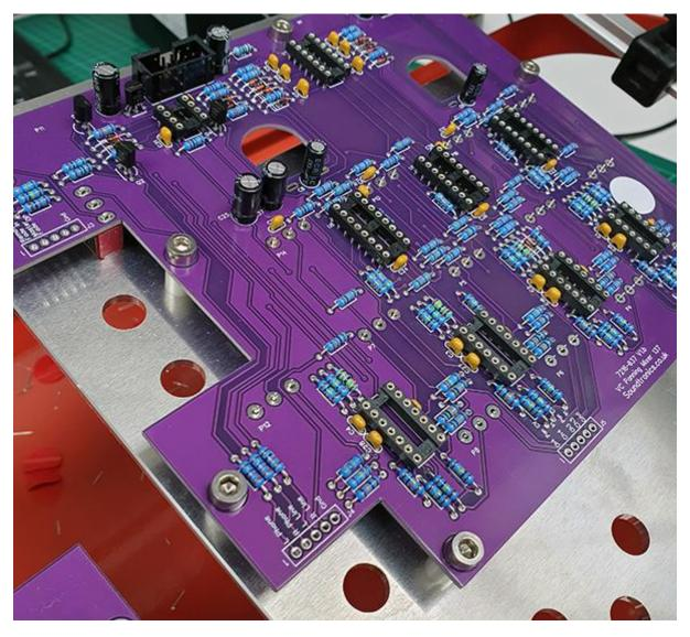
Step 5 – Solder the pots, switches & LEDs. Make sure the toggle switches are lying flush on the aluminium. The LEDs + spacer are to be flush to the PCB by puling the LED upwards using one of its legs while soldering the other leg.
