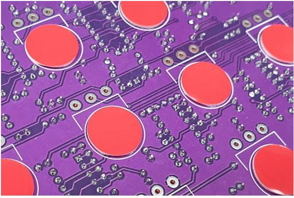
Step 2 – Remove the backing paper from the pad, tweezers are useful for this and place the respective pot in its correct location/ Most pots are B100k but not all! Do not solder at this time.
